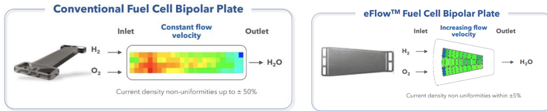
Figure 1: Conventional vs. eFlow™ Fuel Cell Bipolar Plate
